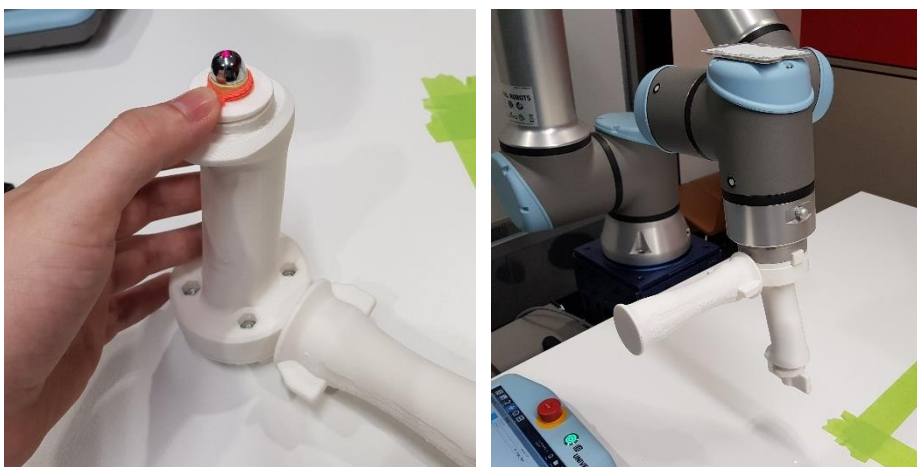
Figure 5: 3D-printed plastic hand-guiding tool with insertable laser to indicate position on path
