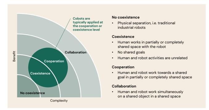
The level of collaboration is forecast to change as we seek to move up the value chain and deploy cobots in more Australian workplaces. To facilitate this change, we need to better understand the relationship between humans and cobots (including physical and mental impacts on employees using cobots) to produce optimum outcomes for business performance and employee wellbeing. Without this understanding, there is a risk that industry and employees may delay or under-utilise cobots.
