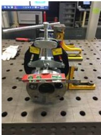
Figure 3.a: Front view of traditional flange-to-pipe alignment showing traditional pipe-clamp and traditional spirit level being used.
