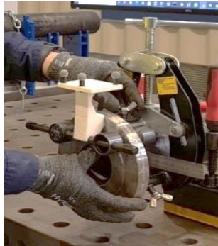
Figure 4.a: Performing flange-to-pipe alignment using digital spirit level in place of traditional spirit level.
