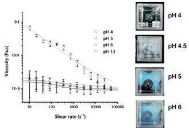
**FIGURE 1** Rheological profiles of fatty-acid terminal silica nanoparticle dispersions at different pH values
