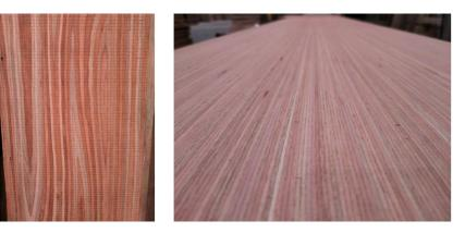
Figure 1. Variable patterns can be achieved through process parameter changes, here in Red Mahogany (image width 250mm)
