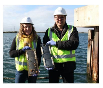
Figure 1. Biofilm formation on conducting coatings after 55 days in in Port River (April-June), Adelaide. Control coupon (left) and a coupon exposed to intermittent electrochemical stress (right) during the experiment.
