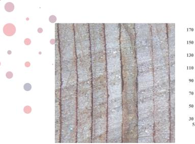
Figure 2. Optical microscope image of product cross-section showing interface between recombined veneers and adhesive, similar to growth rings in timber (image width 15mm)
