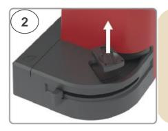
Remove cuvette holder by lifting it straight up.
